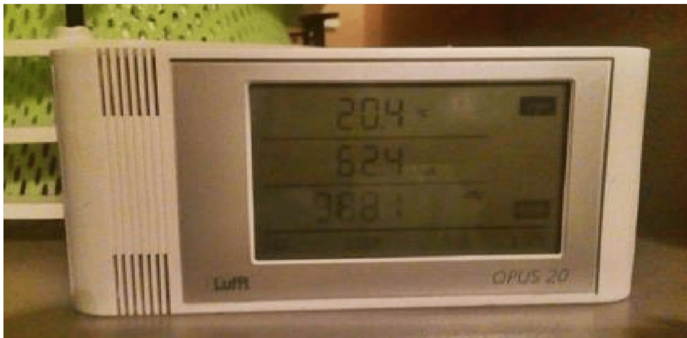
Figure 5: OPUS 20 thermometer and barometer
