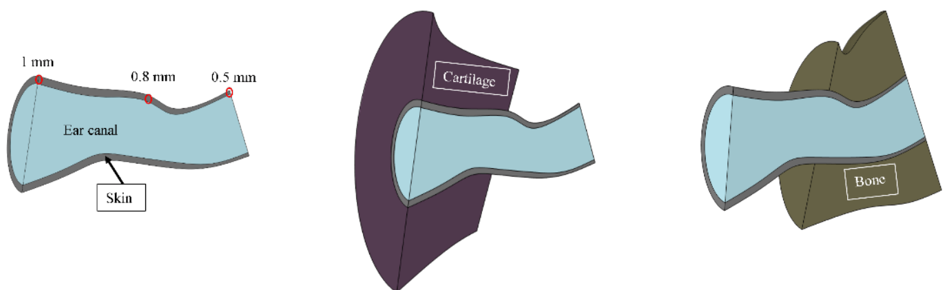
Figure 3. Geometric model and dimensions of (a) the skin, (b) cartilage and (c) bone.
