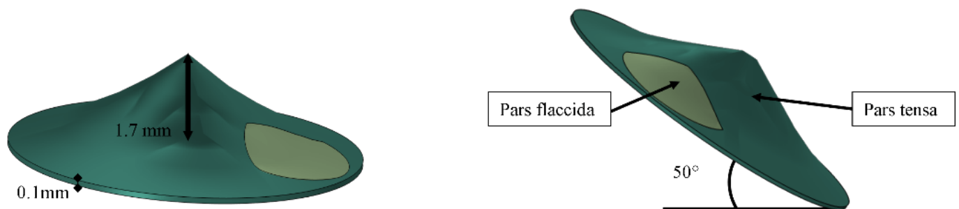
Figure 2. Geometric model and dimensions of the eardrum.
